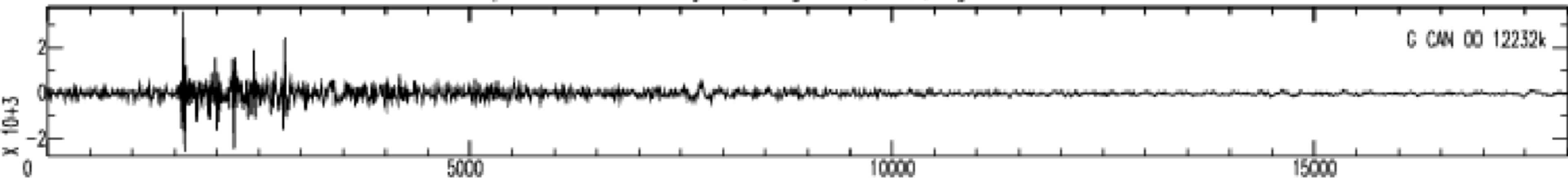
GEOSCOPE Stations/VHZ channel - Time in seconds - 0.002Hz high pass filtered data
