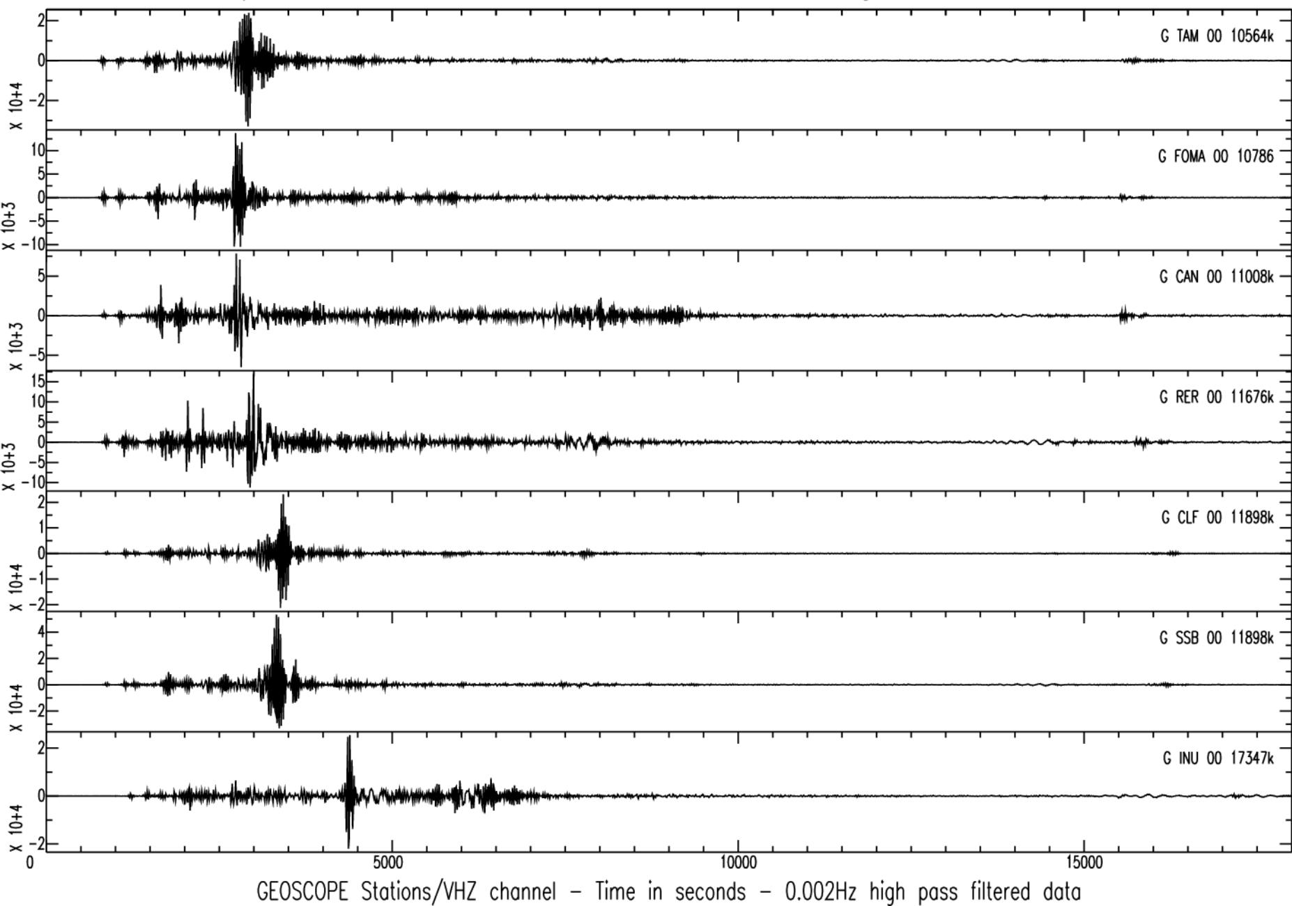
GEOSCOPE Stations/VHZ channel – Time in seconds – 0.002Hz high pass filtered data
